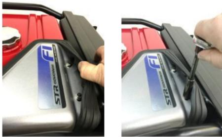
1a-2 /3 Pull back rubber gasket and remove 2 #10mm nuts then pull up and remove corner cover.
