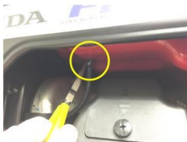
1c-1 Disconnect gas tank vent tube from underneath side of gas tank. No fuel should spill doing this. NOTE: pry down from top vs pulling so as not to rip tube.
