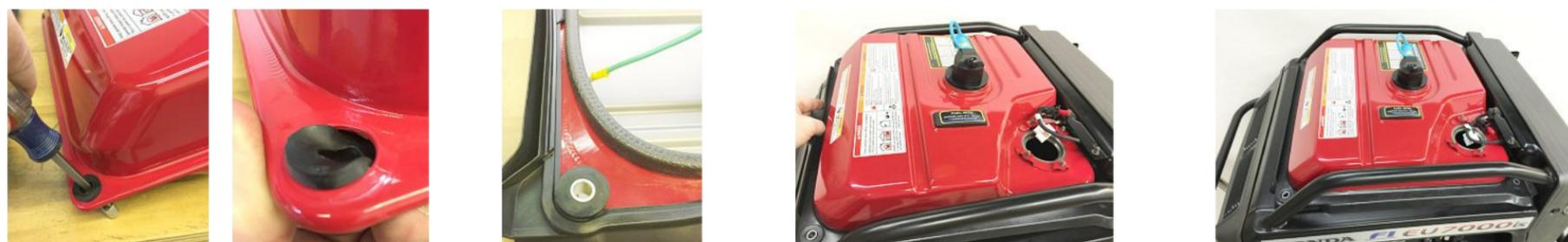
2c-1/2 remove gasket and shock isolators from removed gas tank.
