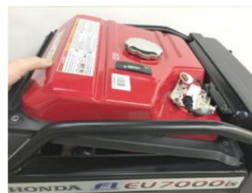
1c-4 Lift back edge of tank - pull back, up and away from back of unit to clear front frame bracket.
