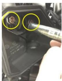
1e-1/2/3 Remove final piece of airbox from throttle body by removing inner two #10mm nuts, loosening clamp below and then swinging plastic box off studs and pulling up.
