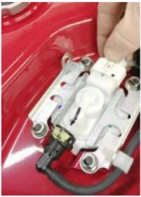
1b-1 Disconnect electrical connector for fuel pump by pressing tab.
