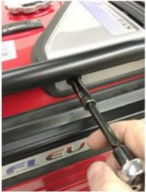
1a-1 Remove #10mm side bolt holding corner cover on
