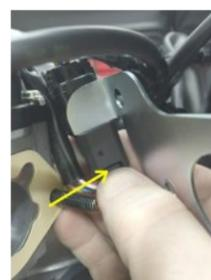
1e-4/5 Remove cable harness support bracket by first removing black plastic push in connector. use pliers to press backside of small push through and pull from other side to release. Then press tab on larger connected and pull down and away. Save gasket after removing from silver plate.
