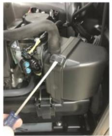
1d-3/4 Remove air box cover by prying up on 4 corner clips then lift off vent tube from top corner.
