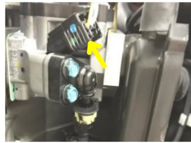
1d-5 Unplug gasoline fuel injector electrical connector. This will prevent the gasoline fuel injector from "dry firing".
