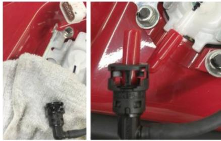
1b-3/4 Catch small amount of any remaining gasoline with small rag and use supplied caps to seal both ends. Push round end in first.
