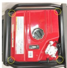
1c-2/3 Locate and remove four #10mm corner bolts with washers then disconnect gas line from white clip on fuel pump bracket.
