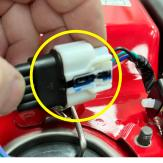
2d-3 Connect Honda fuel pump harness to new fuel solenoid connector under top to generator. Push together until it they <u>click</u> into place.
