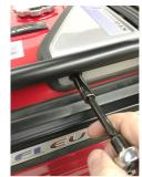
1a-1 Remove #10mm side bolt holding corner cover on
