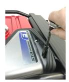
1a-2 Pull back rubber gasket and remove 2 #10mm nuts then pull up and remove
