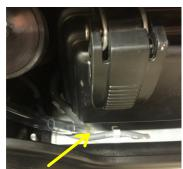
2e-1/2 Route the long clear vent tube (attached to the demand regulator brass fitting under the new top) by routing it behind the latch and lower small 1/4" gray tube. Then push the reduced section through the slot in the floor alongside the existing %" gray tube. The new vent tube should stick out about 34" to 1" below the bottom of the generator. MAKE SURE to not crush these tubes when the generator is in use.
