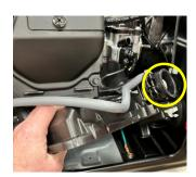
1d-4 Once you get the back half of the air cleaner housing free of the threaded stud, carefully pull the left side out of the cabinet first. Note the fuel line tends to catch on the rubber coupler circled in the picture.
