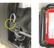
1b-4/5 Locate and remove four #10mm corner bolts with washers then disconnect gas line from white clip on fuel pump bracket.
