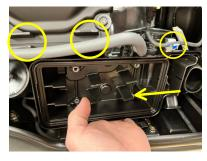
1d-3 Remove the gray tube from its two holding tabs, then remove the fuel line from its white plastic clip, then pull the air cleaner back half directly towards you to free it from the one bottom right threaded stud (arrow). There will be some resistance because the far right side of the housing is still inserted into the front bulkhead.
