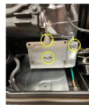
2a-6 Re-install the support bracket and air cleaner back and front half per how they were removed earlier.
