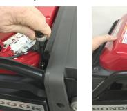
1b-6 Lift back edge of tank - pull back, up and away from back of unit to clear front frame bracket. TIP lift up pull starter side of lid above black handle as you are pulling back.
