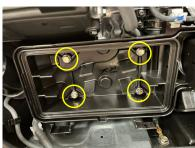
1d-2 Remove 4 fasteners (3 bolts and one nut) holding the air cleaner back half onto engine and save for later.
