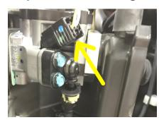
1c-1 Unplug gasoline fuel injector wire harness connector. This will prevent the gasoline fuel injector from getting damaged by "dry firing" while using alternate fuels. Tuck connector in behind throttle body to keep it from bouncing around.
