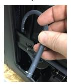
1b-2/3 Gently twist tank vent tube and insert into forward hole on backside of door latch for safe keeping. This will only be needed if you switch back to gasoline.
