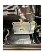
1d-5 Remove the three bolts holding the air cleaner support bracket in place and remove the bracket. Note it will help to keep the bolts in the holes they came from while the bracket is off.
