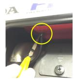
1b-1 Disconnect gas tank vent tube from underneath side of gas tank. No fuel should spill doing this. NOTE: pry down from top vs pulling so as not to rip tube.
