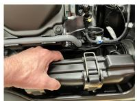
1d-1 Unlatch the air cleaner cover in two places then pull out with air cleaner filter.
