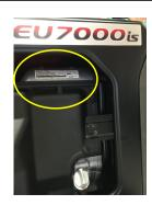
label over existing label at top of engine (inside door).
