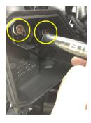
1c-3 Remove the two nuts holding on inner air box and discard. New standoff nut will be put in their place.
