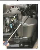
1c-2 Remove air box cover by prying up on 4 corner clips. TIP: Remove lower air filter cover just below air box for better access to bottom two clips. The outer cover and clips are not used anymore.
