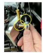
2c-4 Install the aluminum the supplied two #10mm bolts
