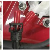
1a-4/5/6/7 Disconnect electrical connector for fuel pump by pressing tab. Then disconnect fuel line fitting from fuel pump by pushing down on yellow tab then pushing in fuel hose quick fitting, then pull out fitting (pushing in first makes release easier). Catch small amount of any remaining gasoline with small rag and use supplied caps to seal both ends. Push round end in first.
