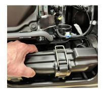
2c-5 Replace the air cleaner cover with the filters inside and latch shut.
