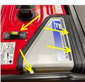
2d-4 Install silver cover over vent section and fasten side bolt and two nuts under gasket. NOTE fuel selection switch location.
