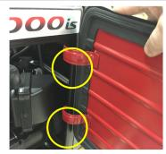
1a-3 Lift off door to gain access to air cleaner side of generator (left side when looking at front)
