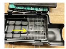
2a-7 Install the Genconnex wire mesh between the plastic air cleaner lid and foam air filter at the front of the filter as shown. This mesh screen is designed to prevent the front edge of the foam element from slipping down into the lid and restrict airflow which would cause the generator
