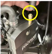
Your generator has been configured to run from either propane or natural gas by way of a removable set-screw orifice installed in the end of the brass tube shown to the left. If you want to change fuel, just replace this orifice with the orifice supplied for that fuel. Remove hose, use supplied 3/8” allen wrench to remove then screw back in the correct orifice, re-attach hose.
